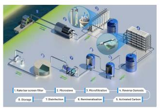
The canal water from the Ostend Canal is treated in 8 stages before being ultimately fed into the region's pipe network as clean drinking water.
